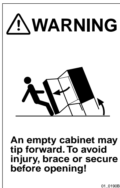
Figure 18 Warning label on the cabinet door
